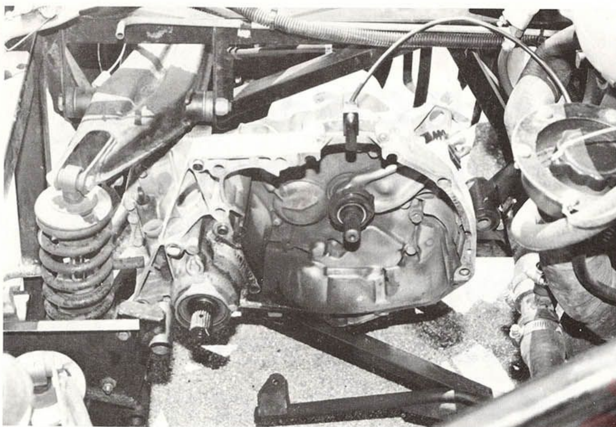
A look at the Sports Renault's transmission housing, engine mount and suspension arms.
